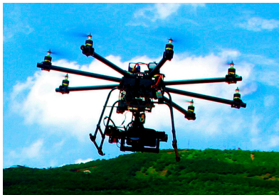
Figure: Eight-rotor UAV platform (BNU-D8-1) fitted with Canon 5DII. Source: [Xu et al., 2014].
